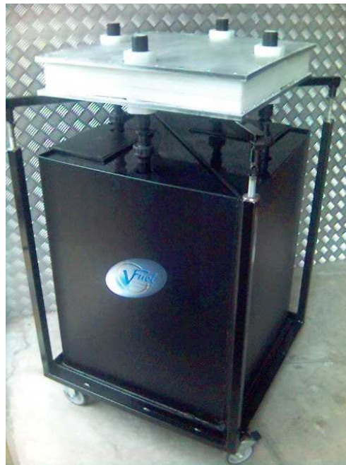
Figure 9: 1-2 kW/6 kWh VRB incorporating V-Fuel's low cost stack design.
