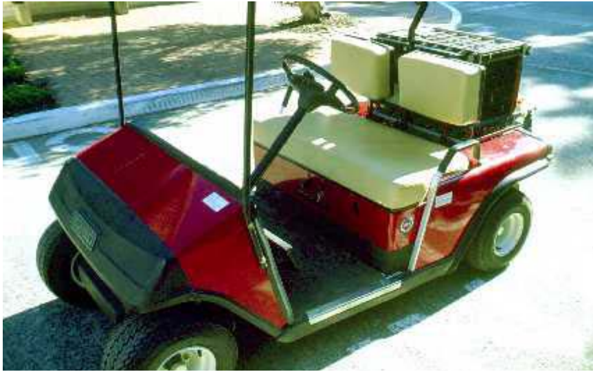
Figure 6: UNSW Vanadium Fuel Cell Powered Electric Golf Cart
